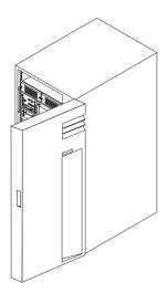
2. Loosen the retaining screws that hold the disk drive cover to the drawer and remove the disk drive cover from the drawer, storing it in a safe place.
